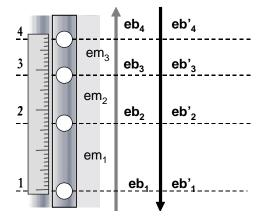
Figura 3: Hole bar errors and machine errors
