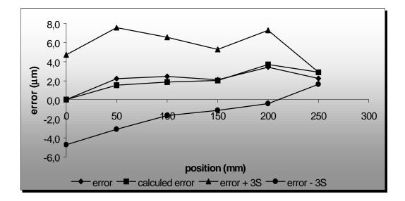
Figure 4: Machine positioning error
