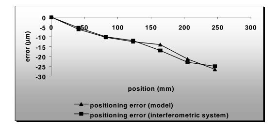
Figure 5: Hole bar positioning errors
